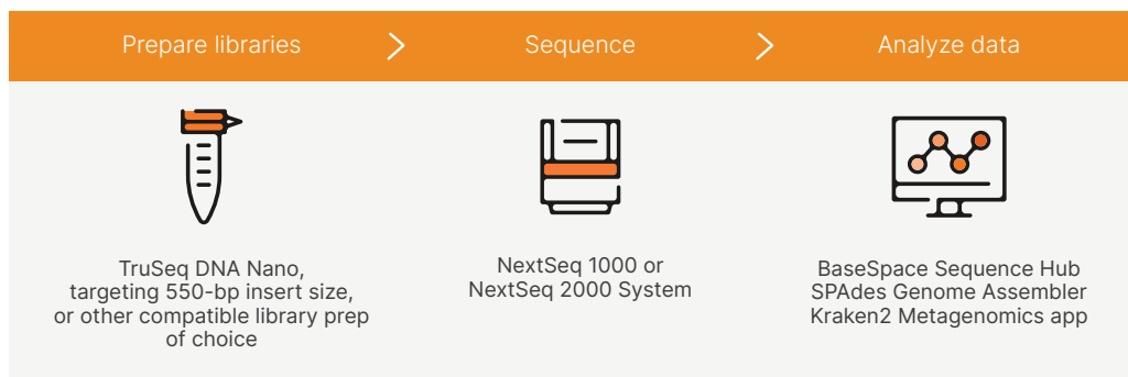
Figure 1: Shotgun metagenomics NGS workflow on the NextSeq 1000 and NextSeq 2000 Systems.
